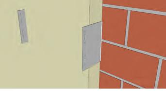
3. Securing angular support profiles to the wall consoles
