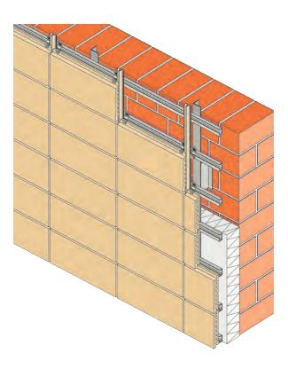
Figure 2 – Horizontal substructure
