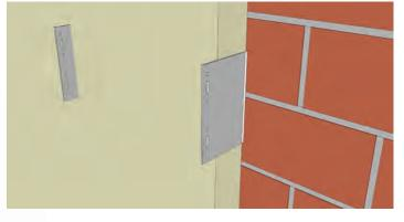
3. Installation of aluminium T-profiles on wall consoles
